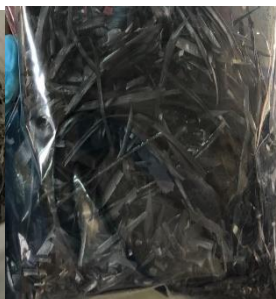
Biochar from sugarcane via pyrolysis
