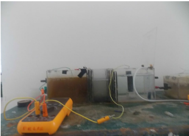
Fig. 2 Laboratory setup of microbial desalination cell
